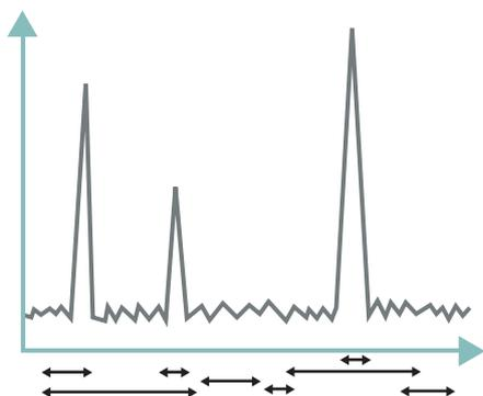
The channels can be reallocated dynamically when running and modifying one channel does not affect the operation of the other ones. The channelized data is output as IQ-data that is sent for analysis with the streaming interfaces.
